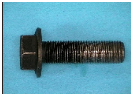
Figure 27. Once the Adhesive is Removed, a Clean Shiny Steel Surface Should Remain
