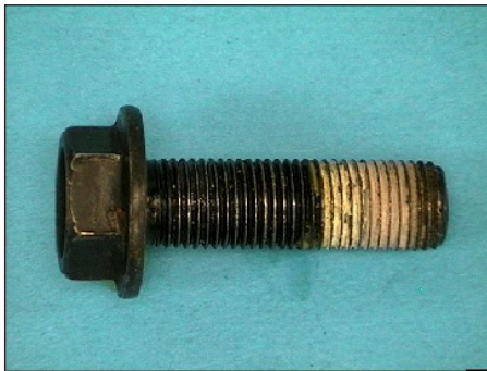
Figure 25. Used Caliper Mounting Bolt with Adhesive Patch on the Threads
